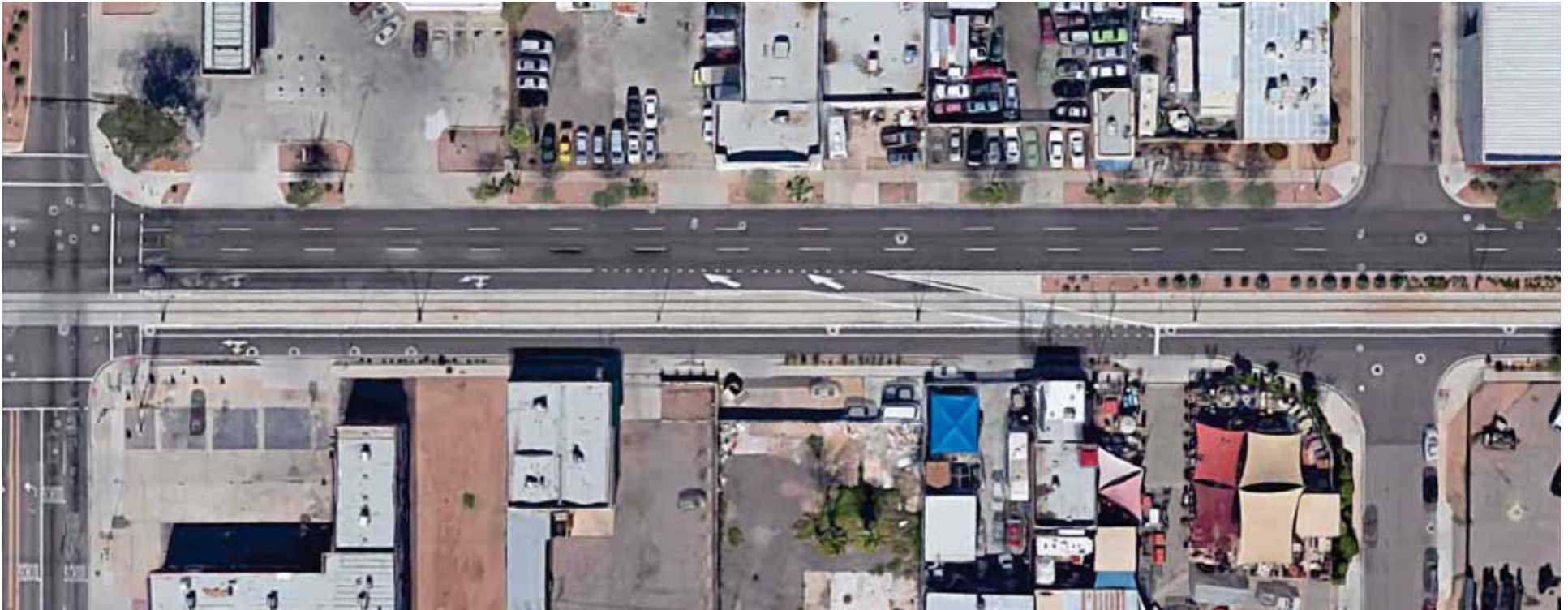
Valley Metro Light Rail in Phoenix uses a unique center alignment on one-way couplets. This section of Washington Street shows westbound traffic lanes on both sides of the light rail tracks, as well as a midblock track crossing for car traffic. This arrangement maintains access to driveways along both sides of the street.
